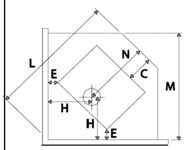
Dimension "C" is taken from front of door seal lip to front edge of floor protector. All dimensions are in millimetres & are set as a "minimum" in accordance with test report 05/1249 under ASNZS 2918:2001.
