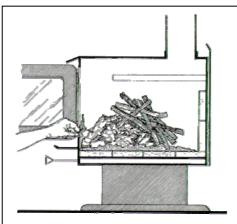
**TO BUILD A QUICK, HOT FIRE** Use plenty of crumpled newspaper and dry, finely-split kindling. Set the air control fully open. Light the newspaper near where the combustion air enters the firebox. When a kindling fire is built properly, you should expect instant ignition and no smouldering.
