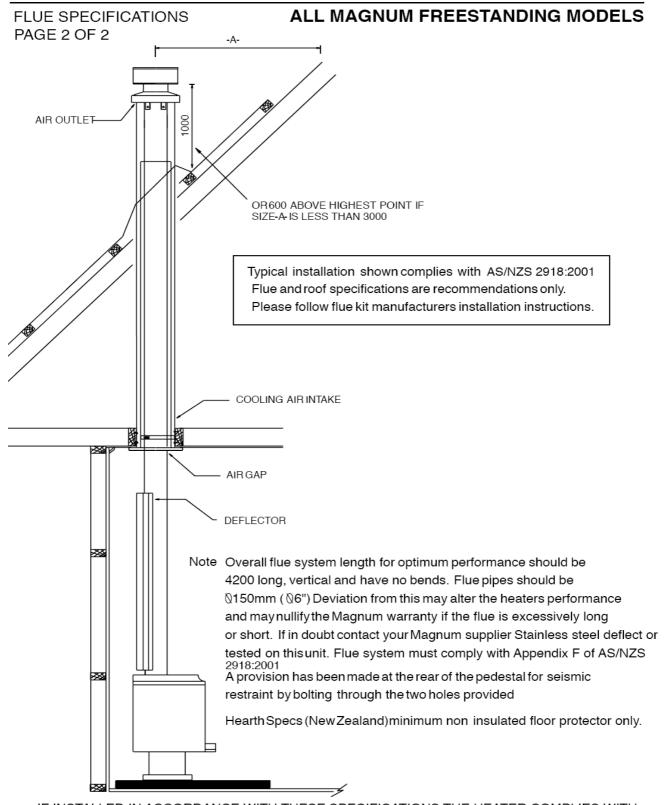
IF INSTALLED IN ACCORDANCE WITH THESE SPECIFICATIONS THE HEATER COMPLIES WITH AS/NZS 2918:2001 including appendix F
